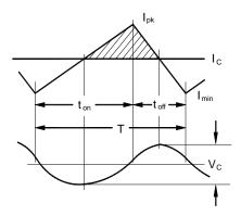
Figure 5. Input Capacitor Voltage and Current Waveforms
