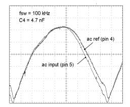
Figure 2. AC Ref with Phase Delay
