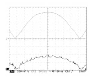
Figure 4. Current Shaping Loop Oscillations
