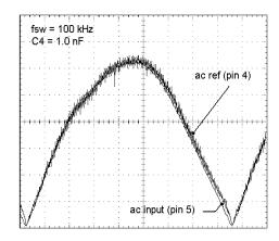
Figure 3. AC Ref with Minimal Phase Delay
